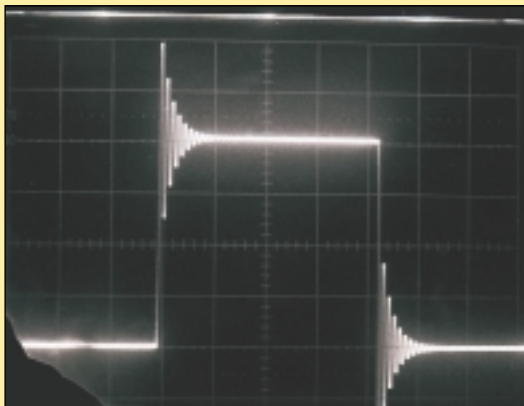
Square Wave Response Frequency: 1 kHz (8 \Omega /2 \mu F capacitive load)
